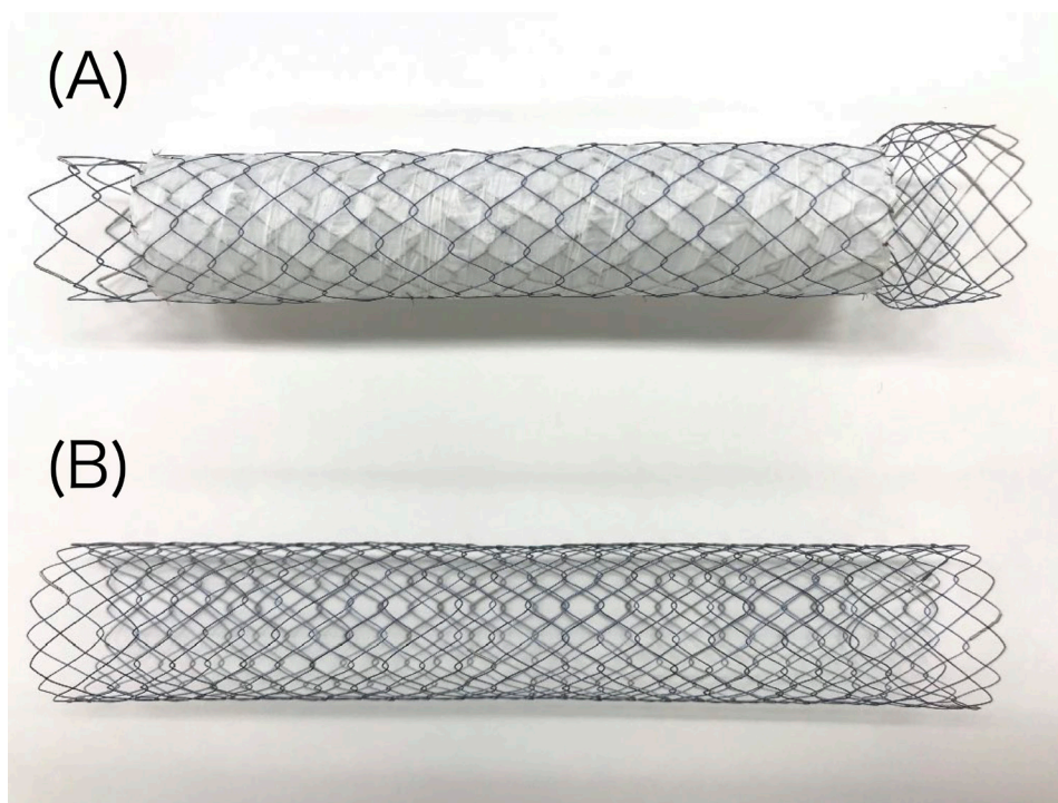
Figure 1 Covered and uncovered self-expandable metallic stent (SEMS) used in this study. (A) The covered SEMS has an antimigration system at both ends (proximal uncovered flare and distal uncovered area). (B) The uncovered SEMS is straight and contains no membrane.
